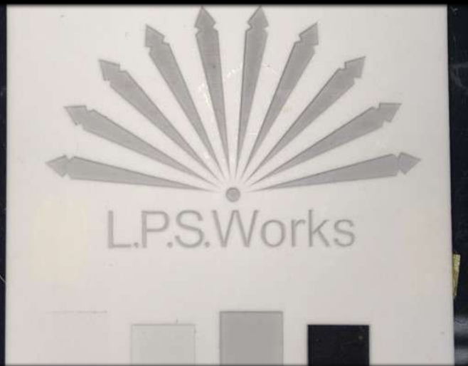
Alumina Ceramic Spot-Facing Processing Depth: 340 \mu\text{m} / Plate thickness: 380 \mu\text{m}
