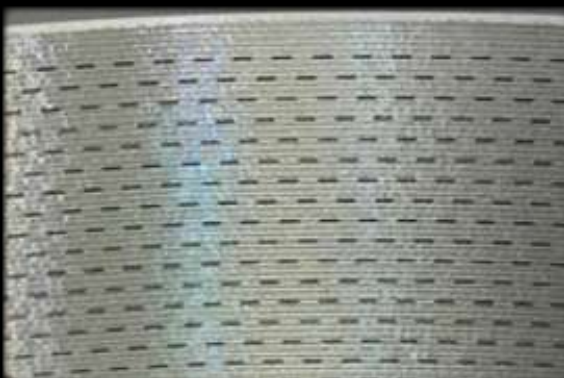
Groove Width of 30 \mu\text{m} : Broken Line Processing
